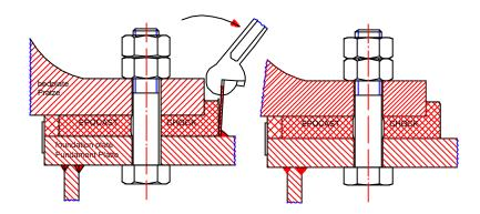
**2.5.4.** Remove the bolt plugs and insert the bolts. Ensure the chocks cool to ambient temperature before tightening the holding down bolts in accordance with instructions.
