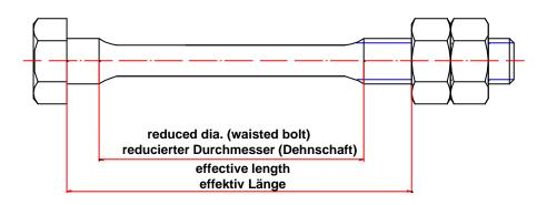
**3.14.** To find the bolt torque from a given tension:-
