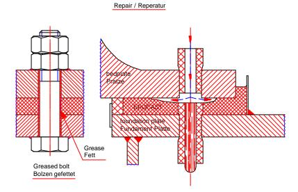
2.8.2. Sometimes a vertical crack occurs running into the bolt hole. This can be left, but for aesthetic reasons it is usual to grind out the crack to about 30 mm and pour in new **EPOCAST 36** to repair the crack.
