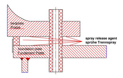
2.2.12. For generators, deck machinery and small units you may apply a thick coating of thick high melting point grease to the holding down bolts before inserting them. These bolts should only be hand tight. If chock thickness exceeds 50 mm then follow instructions for larger units in the next paragraphs. Where possible use foam plugs in preference to wood plugs or bolts.
