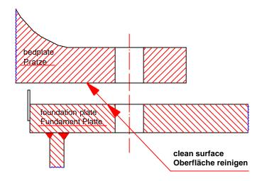
2.2.7. Flexible damming is inserted between the bedplate and foundation to form liquid tight sides for the moulds or dams. Make sure the damming is firmly in place, and cannot collapse or leak. The EPOCAST exerts a surprisingly strong pressure on the lower edge of the damming. So take extra care when forming dams.
